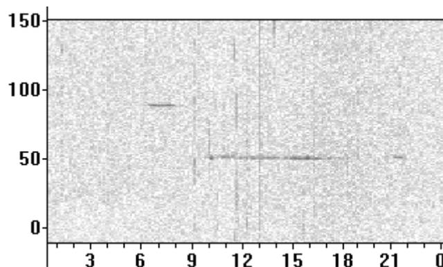
Fig 6. Waterfall of sounder in Northern Australia received in UK on 16MHz, showing morning longpath at 89mS and afternoon shortpath at 50 mS.
