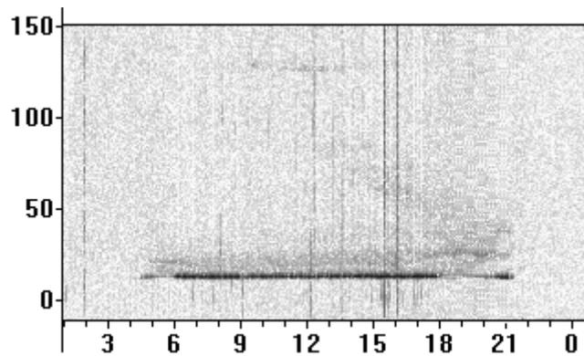
Fig 8. Waterfall of Cyprus sounder received in UK on 29MHz, with the direct path at 12mS some sidescatter paths, and brief traces of longpath at 127mS.
