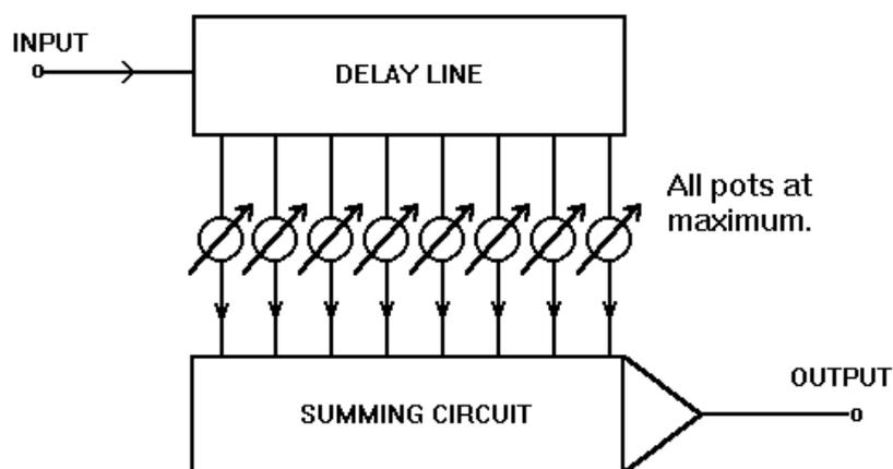
Fig 2. Simple low-pass FIR filter with delayline with a potentiometer on each stage and a summing circuit to form the output.
