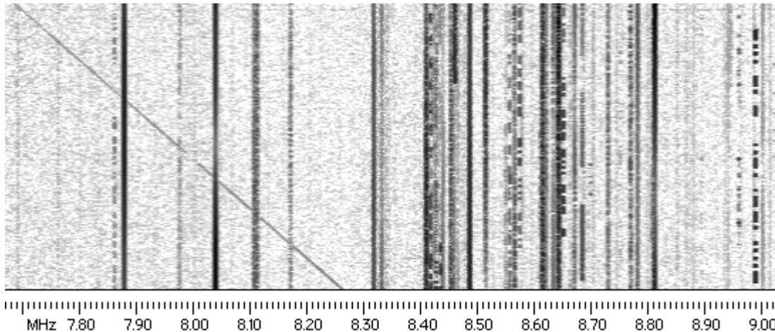
Fig 1. Spectrogram showing sweep sounder passing 8 MHz. The vertical axis represents about 5 seconds.
