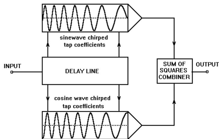
Fig 4. Final chirp filter consisting of one delay-line, two sets of chirped sine/cosine tap coefficients, two sum-of-products circuits and a sum-of-squares combiner.
