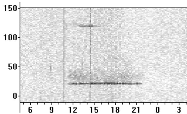
Fig 7. Waterfall of sounder in the Eastern USA received in UK on 21MHz, showing the direct path during the day at 21mS with simultaneous long path at 118mS in the afternoon.
