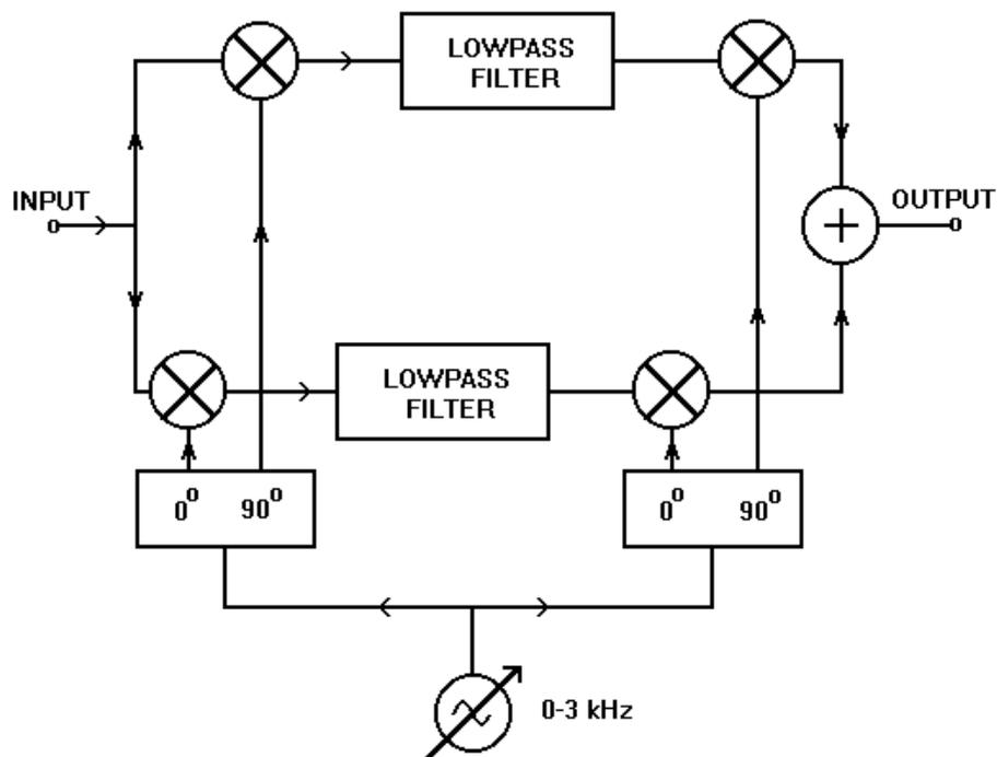
Fig 3. Tuneable bandpass filter made from two of the filters of Fig 2, built into an image-cancelling down-up converter.
