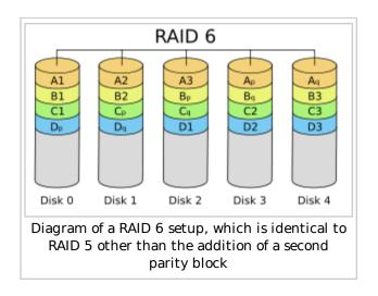
it is possible to extend the approach to produce redundancy simply by producing another syndrome; typically a polynomial in  $\mathbf{GF}(2^8)$  (8 means we are operating on bytes). By adding additional syndromes it is possible to achieve any number of redundant disks, and recover from the failure of that many drives anywhere in the array, but RAID 6 refers to the specific case of two syndromes.
