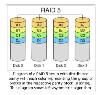
mdadm in Linux. A minimum of 3 disks is required for a complete RAID 5 configuration. In some implementations a degraded RAID 5 disk set can be made (3 disk set of which only 2 are online), while mdadm supports a fully-functional (non-degraded) RAID 5 setup with two disks - which function as a slow RAID-1, but can be expanded with further volumes.
