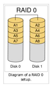
In the diagram to the right, the odd blocks are written to disk 0 while the even blocks are written to disk 1 such that A1, A2, A3, A4, ... would be the order of blocks read if read sequentially from the beginning.
