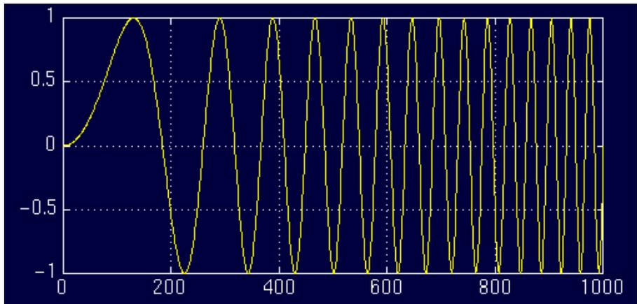
Figure 6: Chirp waveform
